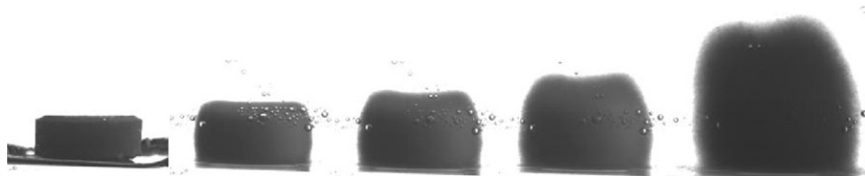
Fig. 3. Images of a dry HPMC compact and the same compact after swelling for 30 min, 1 h, 6 h, and 15 h. The dry compact diameter is 10.3 mm.
